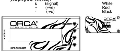
Connect the battery wires to a charged pack of battery. Turn on the ESC and the setting card will activate automatically. Note that the screen will show "Loading..." during initialization – indicating that the ESC is copying the current setup in the ESC to the setting card. Once loading is completed, the screen will show "TEAM ORCA Program" and Current Firmware Version and Data code e.g. Ver3.0 1XXXXA. You can now start to program your ESC.
